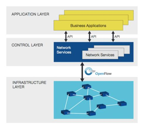
Nothing about management - some management operations are supported by the OpenFlow protocol, OF-config added for control plane setup
